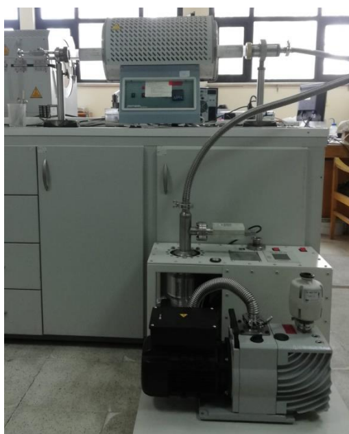
Figure 3.7. Vacuum thermal dealloying setup
