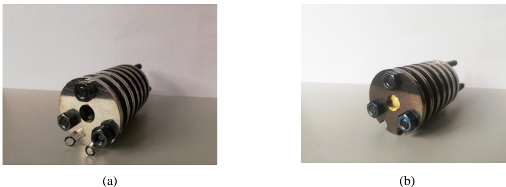
Figure 3.8. Stainless steel mask for vacuum dealloying (a) bare, (b) loaded.
